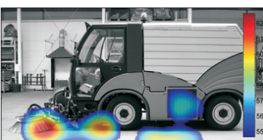
Localized sound sources of a cleaning machine
