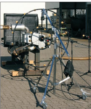
Localization of sound sources on a screw-type compressor using a double-circular array
