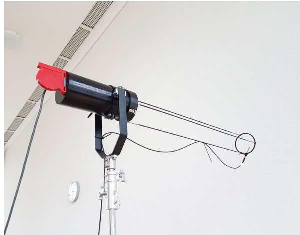
Indoor measurement of the sound absorption coefficient of a wall absorber in situ with AcoustiAdrienne
