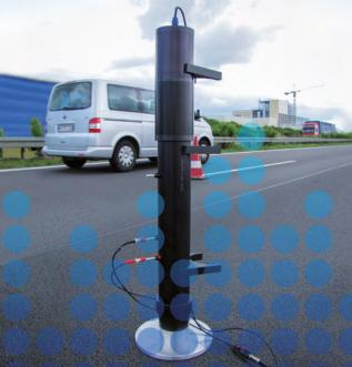
Measuring system AED 1000 – AcoustiTube® for determining the sound absorption coefficient, the reflection factor and the impedance ratio
