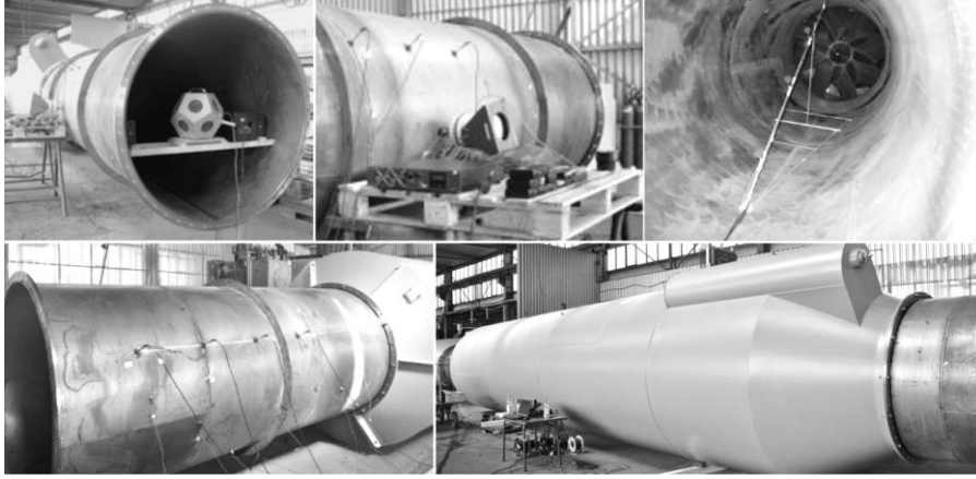
Fig. 7 – Transmission loss measurement of the maritime absorption silencer system under laboratory conditions
