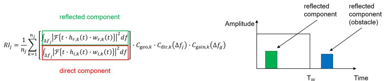
Figure 1.3: Left: Calculation procedure for determining the sound reflection index RI; right: isolated reflected component as a result of subtracting the impulse responses with and without test specimen.
