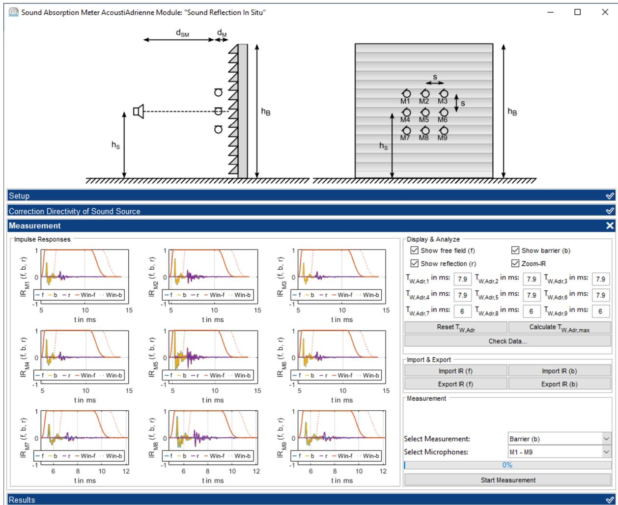
Figure 4.3: User interface of the module Sound Reflection in situ after the full set of measurements is completed and the reflected component has been calculated
