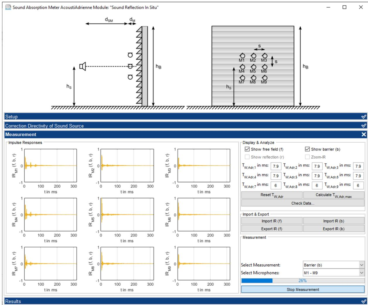
Figure 4.1: User interface of the module Sound Reflection in situ during the measurement of the impulse responses
