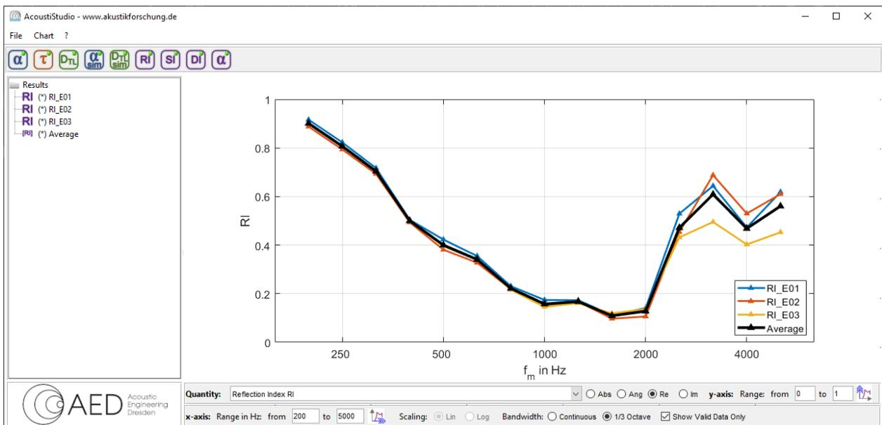
Figure 6.1: User interface of the data viewer of the AcoustiStudio with exemplary measurements of the Sound Reflection Index of three different elements of the same noise barrier and the according average value.
