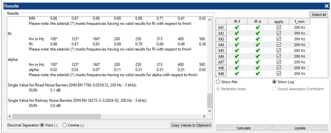
Figure 5.2: Segment of the user interface of the module Sound Reflection in situ with the results as a log-file including the single values DL<sub>RI</sub>
