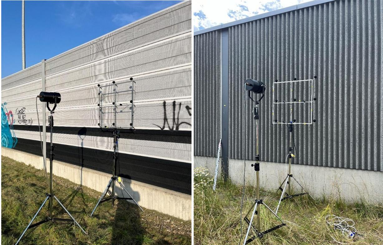
Figure 2.3: Exemplary setups of the measuring system AcoustiAdrienne - module Sound Reflection in situ on noise barriers
