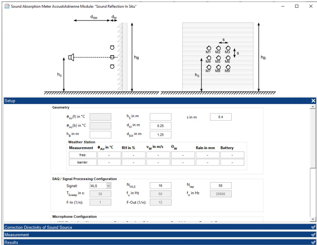
Figure 3.2: User Interface of the module Sound Reflection in situ after starting the software
