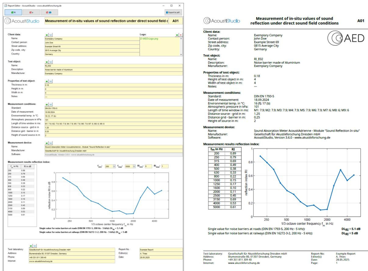
Figure 6.2: User interface of the report generator and exported measurement report for an exemplary measurement of the Sound Reflection Index with the measuring system AcoustiAdrienne and the software AcoustiStudio – module Sound Reflection in situ
