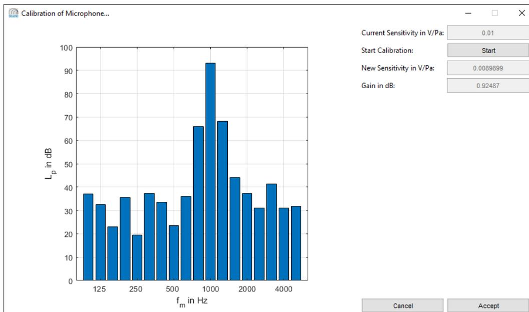
Figure 3.3: dialog window for the calibration of the microphones
