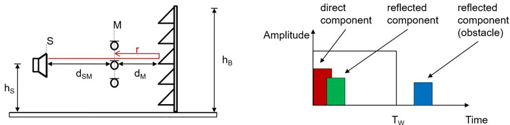
Figure 1.1: schematic measurement setup for the measurement at the test specimen (left) and general result (right)
