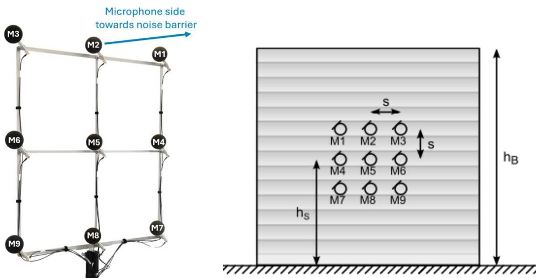
Figure 2.2: Left: Microphone grid with indication of the alignment to the noise barrier; right: schematic representation of the microphone positions from the viewing direction of the sound source
