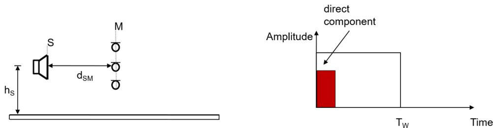
Figure 1.2: schematic measurement setup for the free field measurement without test specimen (left) and general result (right)
