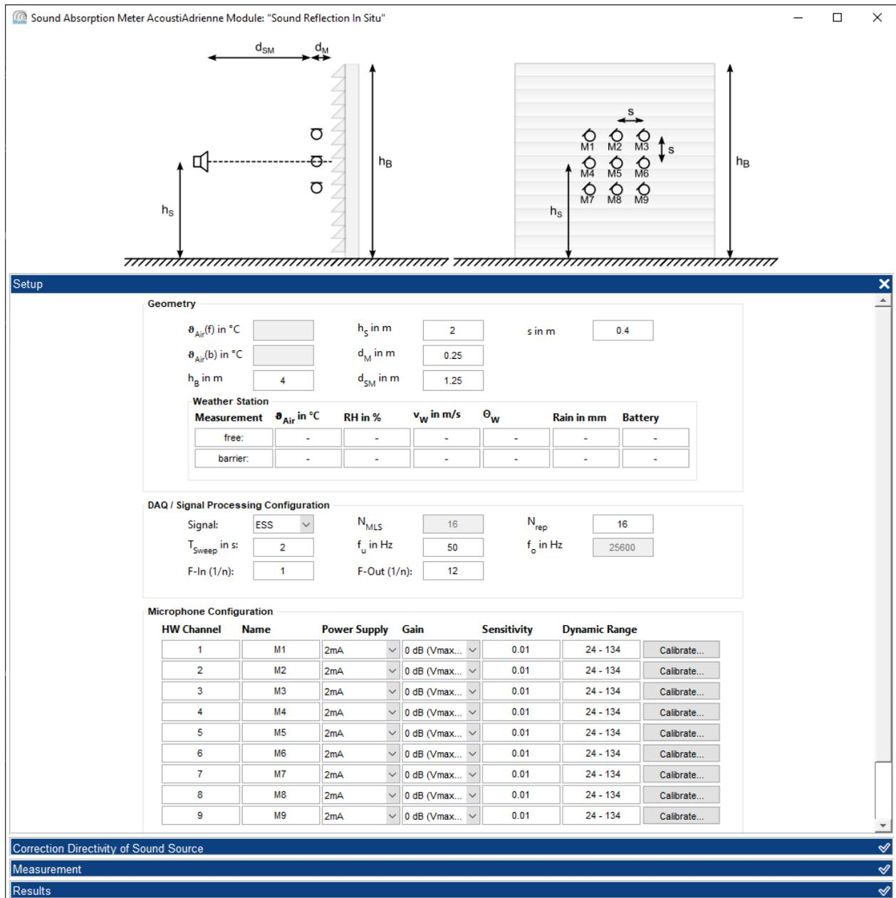
Figure 3.4: user interface of the module Sound Reflection in situ with completed setup page
