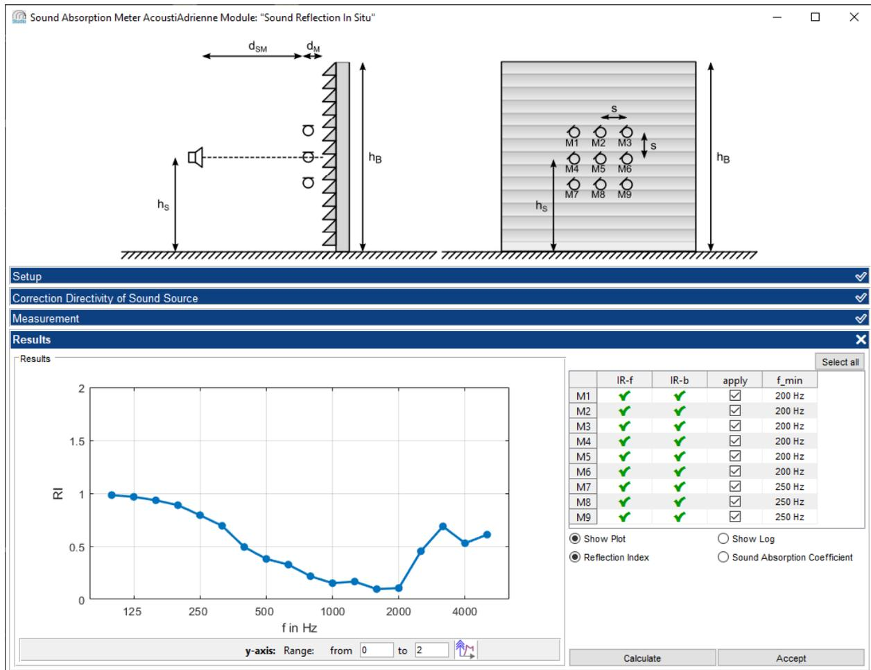
Figure 5.1: User interface of the module Sound Reflection in situ with the graphical representation of the results of an exemplary measurement
