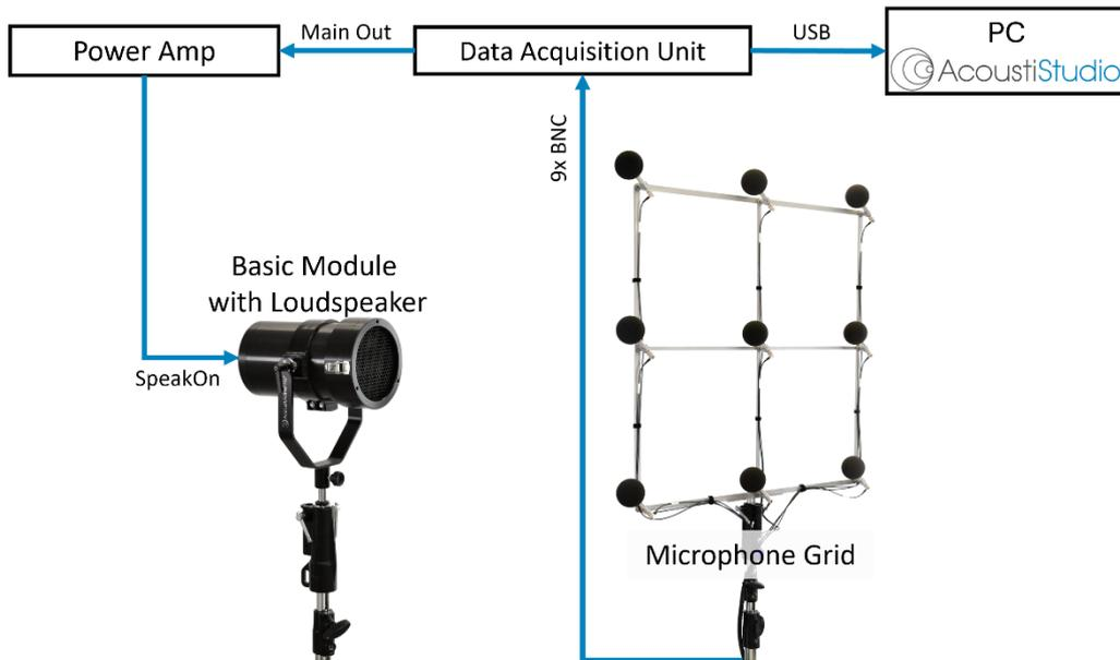
Figure 2.1: schematic setup of the main components of the measuring system AcoustiAdrienne – module Sound Reflection in situ
